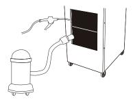
• Cleaning of heat-exchanger: Clean dust attached to the heat-exchanger with compressed air or a vacuum cleaner.
