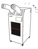
After cleaning, dry well the inside by blowing operation for 3~4 hours.
