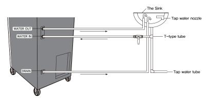
5. Once the pipe connection is finished, open the valve of water supply line so that water is supplied. At this time, as water is discharged only when the air-conditioner is operated, check whether water is discharged from the drain hole.
