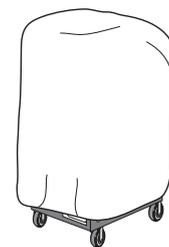
3. Keep machine suitably covered to prevent damage by damp, humidity and dust.
