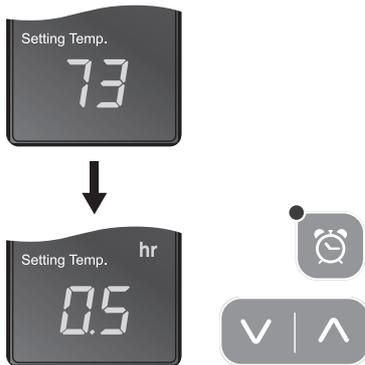
1. When unit is operating, press the 'Off Timer' button and set the length of time you want by pressing  $\wedge$  or  $\vee$ . Each time you press the button you will increase the 'time to off' period by 30mins. up to 10 hours, and 1 hour up to 24 hours. The display will show 5 for 30min and 1 for an hour. One and a half hours will show 1.5.
