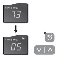
When unit is operating, press the 'Off Timer' button and set the length of time you want by pressing ∧ or ∨. Each time you press the button you will increase the 'time to off' period by 30mins. up to 10 hours, and 1 hour up to 24 hours. The display will show 5 for 30min and 1 for an hour. One and a half hours will show 1.5.
